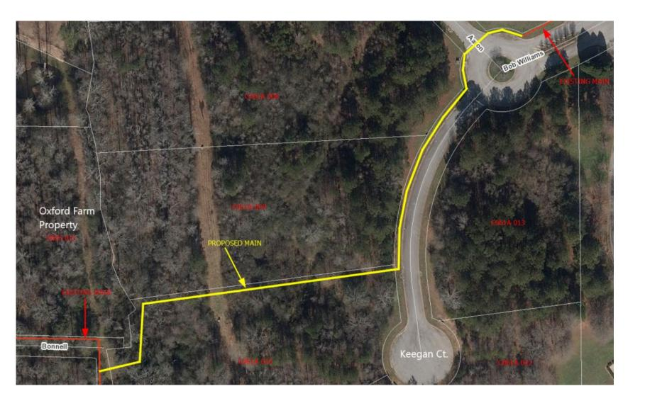
Typically, a utility line alignment would adhere to the property line to preserve the largest developable footprint. But since the City of Oxford owns all these properties (see next slide), a different alignment would be appropriate.
